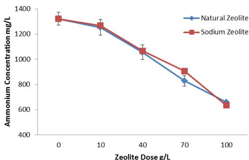
**Figure 3: Ammonium concentration inside the digesters with natural and sodium zeolites at different doses**
