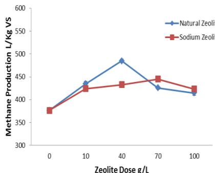
**Figure 2: Methane production with zeolite Dose**
