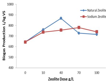
**Figure 1: Biogas production with zeolite doses**
