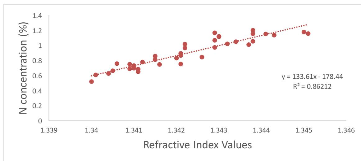
**Figure 1. Calibration curve of N concentration measured in the laboratory versus refractive index values from the urine sensors for urine samples collected from grazing dairy cows.**
